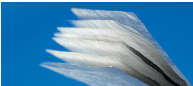
Super-insulation for cryogenic applications. © RUAG Space GmbH
