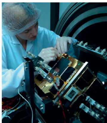
Thermal vacuum testing of the assembled spacecraft. © TU Graz
