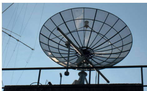
Ground station antenna. © TU Graz
