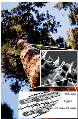
Wood as an example of a natural lightweight nanocomposite for large structures. It exhibits a hierarchical architecture and sophisticated structure on the nanometre scale. © BOKU Vienna
