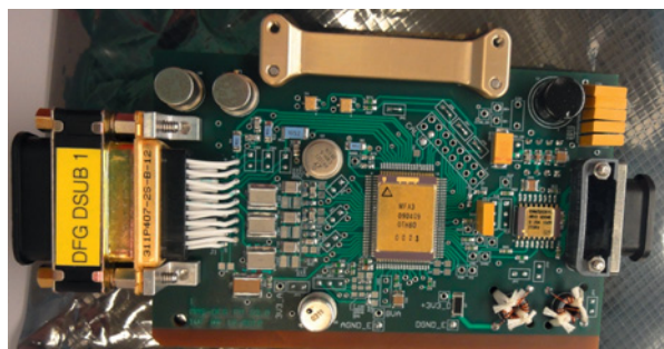
Flight Model of DFG electronics with Magnetometer Front-end ASIC in the middle (chip with golden lid). © ÖAW/IWF
