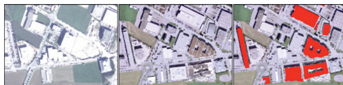
Change detection (left to right: orthophoto 1999 – orthophoto 2008 – recognized changes). © GeoVille, State of Tyrol
