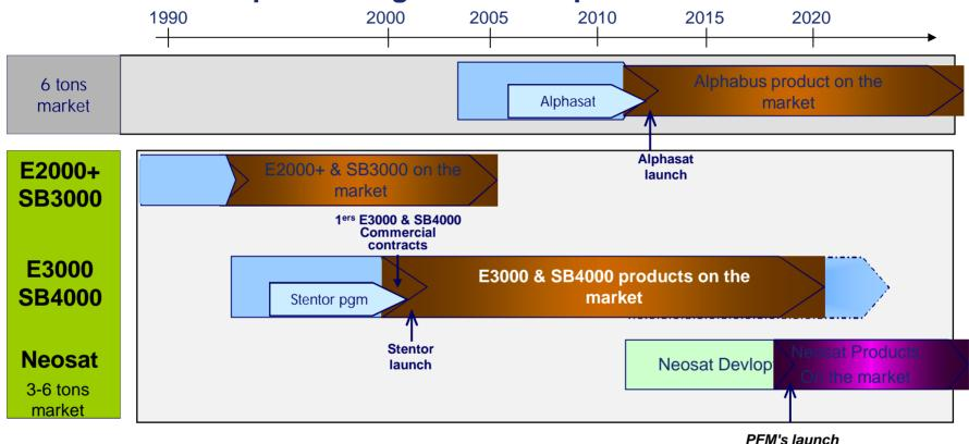
The Eurostar E3000 and Spacebus SB4000 product lines will remain the Astrium and TAS work-horses until Neosat products are commercially available and flight proven.
