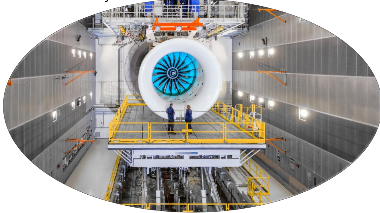
Ultrafan: ducted UHBR engine
