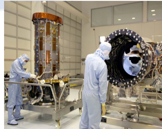
Flight telescopes undergoing integration in Thales Cannes premisses.
