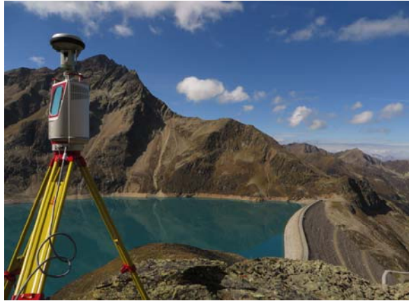
Fig. 1: Terrestrial Lasers-canner (© alpS/Fey).
