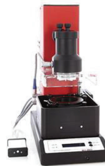
Fig. 1: Tissue softness analyzer (TSA) by Emtec
