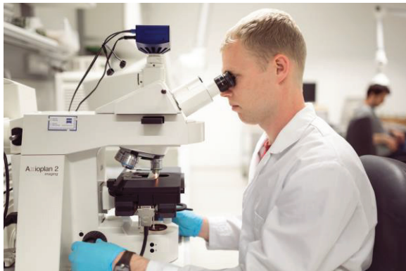
Fig. 1: Examining adhesive distribution by means of fluorescence microscopy (Wood K plus)]
