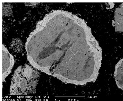
**Fig. 2: Ash layer through interaction between biomass ash and bed material (copyright: BIOENERGY 2020+)**
