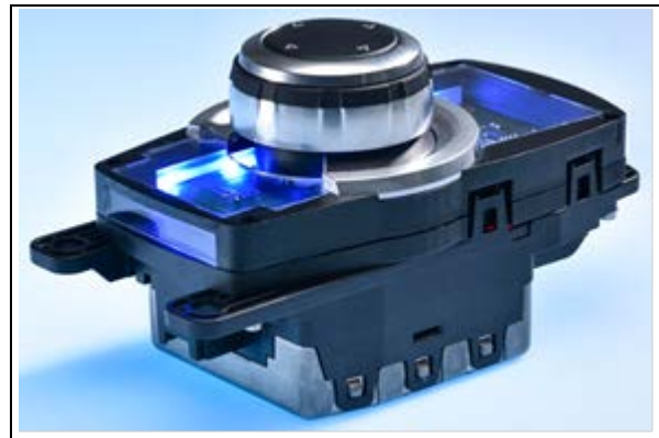
Fig. 2: Final version of the mass demonstrator by integration of the developed magnetic system into a BMW iDrive chassis.
