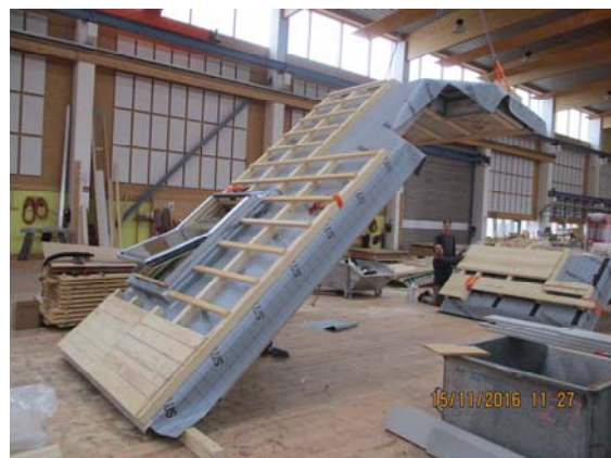
Fig. 1: prefabricated attic extension module (© Graf Holztechnik)
