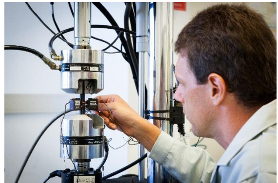
Fig. 1: The Cyclic CRB Test (PCCL)
