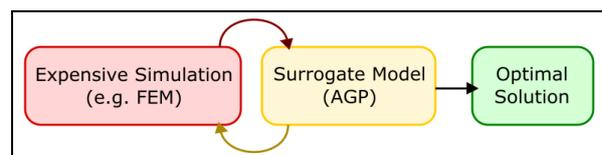
Fig. 1: Flow chart of the optimization approach based on surrogate models.
