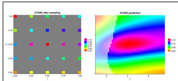
**Fig. 2: Right plot shows the AGP prediction based on the 25 sampled FE data points shown in the left plot. The shaded region defines parameter settings where the amplitude is too small.**
