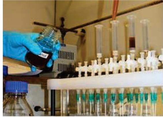
Fig. 1: Loading of the solid phase with a process effluent sample
