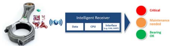
CBM Condition Based Monitoring System (© LEC GmbH)
