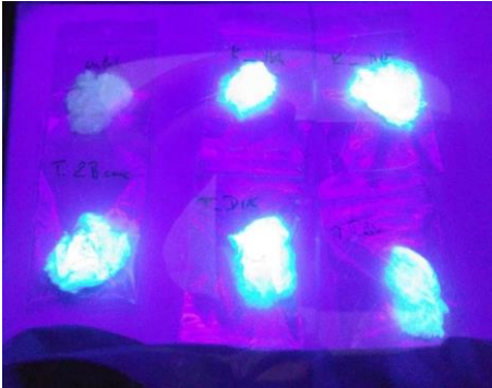
UV light recordings of optically brightened viscose samples after 10s at 210 °C (©Wood K plus)
