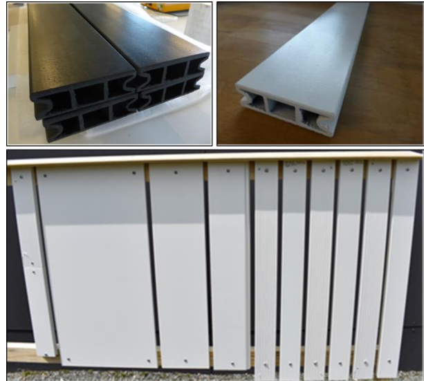
Figure above: Modified wood plastic composite profiles untreated (left) and powder coated (right); Figure below: Wood plastic composite profiles and weather-resistant wood fiber composite boards in natural weathering (test facade) (©Wood K plus)
