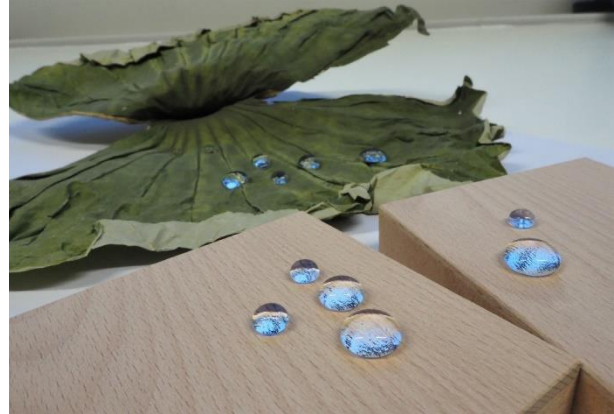
Water drops on the biological role model, a lotus leaf, and on superhydrophobic wood (©Wood K plus)
