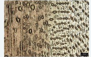
IN718 wall + 1vol% Al_2O_3 , cross section of the IN718 with embedded Allumina
