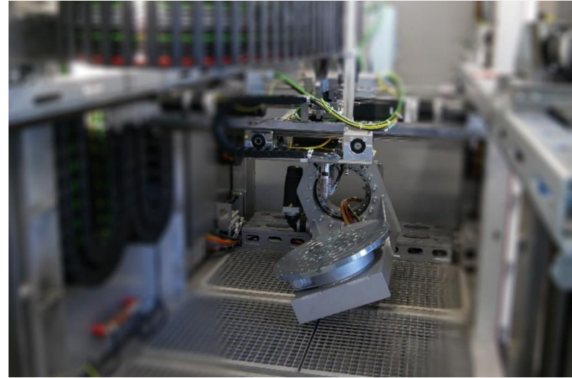
PMD printing station
