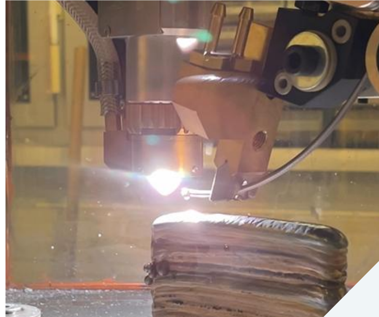
(Torch-system developed by INO in collaborative project GEPROBA, https://projekte.ffg.at/projekt/4762069 )
