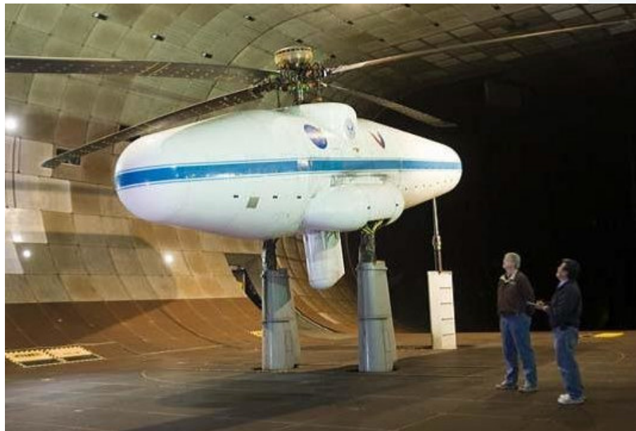
Windkanal NASA Ames: Large Rotor Test Apparatus (LRTA) Sikorsky UH 60 1:1
