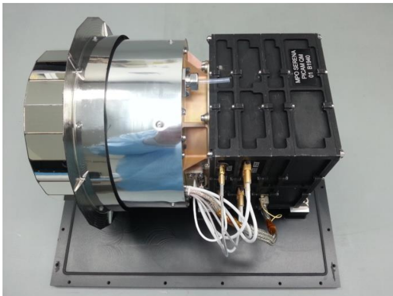
PICAM Qualification Model in its final configuration, mounted on the transport plate.
