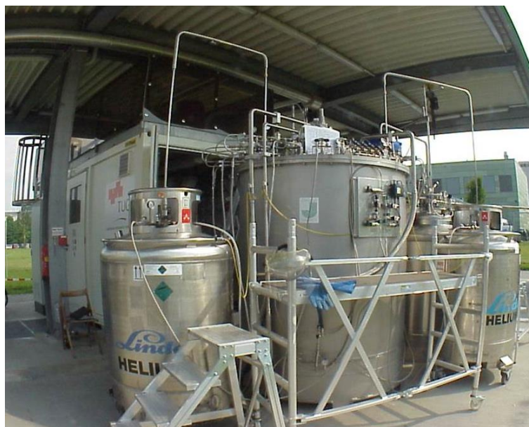
Pilot slush production plant (250liter/hour)
