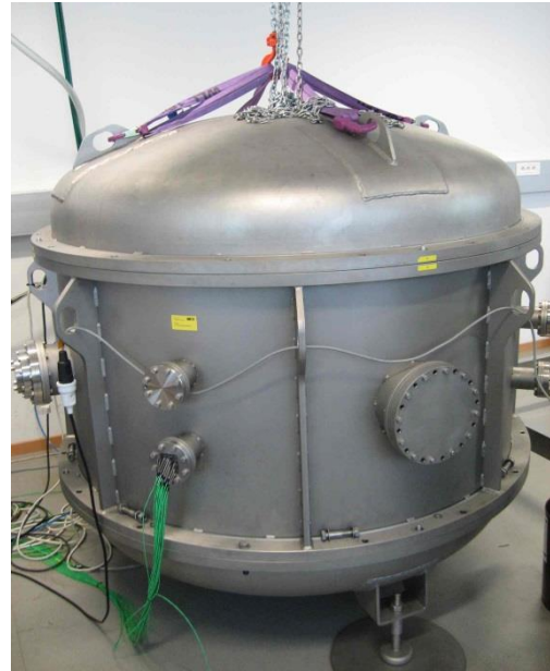
Left: Thermal vacuum chamber (TVC, diameter 0,7m) attached to a clean room class10000. Right: New Large thermal vacuum chamber (LVC; diameter 1,3m) installed in 2013.
