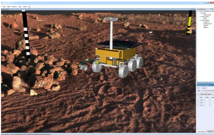
Figure 8: Virtual rendering of PanCam 3D vision processing result (data captured during a field trial at the CNES rover test environment SEROM in Toulouse) with an early ExoMars rover model as well as a scale bar inserted.
