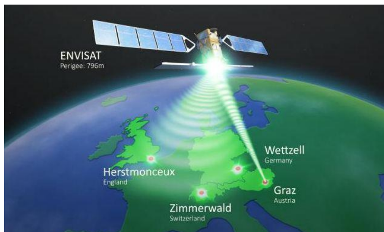
Multi-static experiment: the passive SLR stations in Wettzell, Zimmerwald and Herstmonceux were able to receive photons emitted in Graz (Credits: AIUB).
