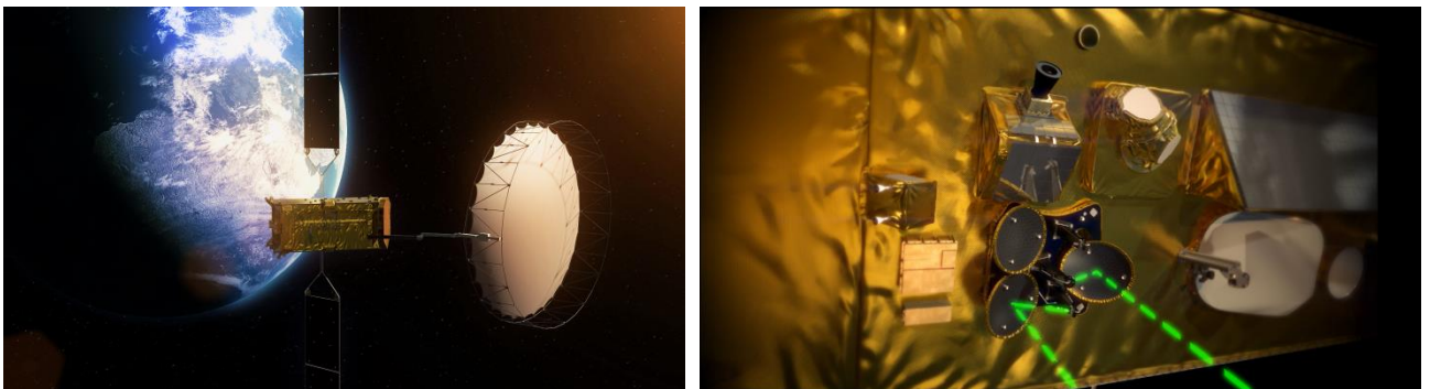
Figure 5: Left: Artist impression of the Alphasat with the big reflector of the main payload from Inmarsat. Right: TDP#5 payload on Alphasat with the three spot beam antennas. Two are focused on Italy sites and one towards Graz. Both © ESA
