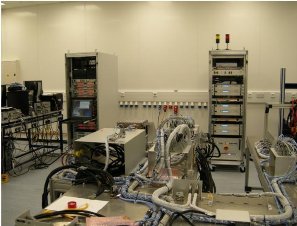
Solar Orbiter Sim FE (left) and the Solar Orbiter Power SCOE (right) in the Astrium UK clean-room
