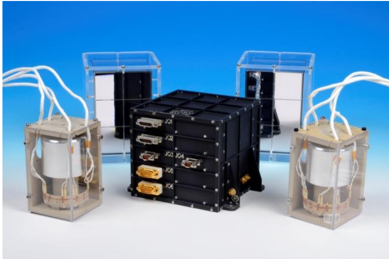
A MERMAG-P Flight Model with electronics box (center), two fluxgate sensors (front right and left) and two thermal protection covers for the fluxgate sensors with highly reflective mirrors (background right and left).
