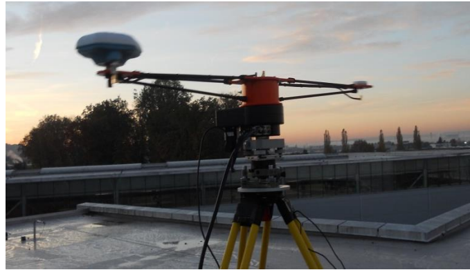
Rotating antenna at the roof of the IWF building. An artificial reflector realized by a copper plate was installed to generate multipath effects in addition to these ones caused by the “natural” environment.
