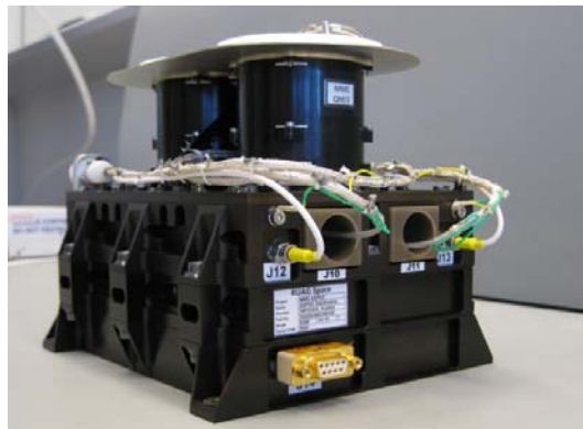
One of the Flight Units (FM). Each FM is equipped with four ion sources
