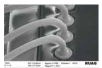
Electron microscope image of bonding detail.
