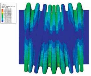
Axial and lateral eigenfrequencies of bellows
