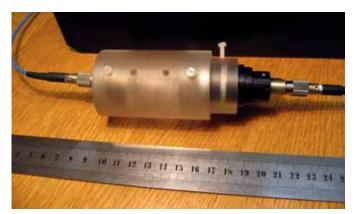
Current CDSM sensor unit (TRL 3 standard)
