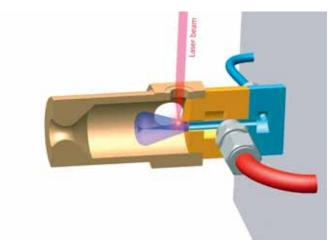
Conceptual view of a test chamber for laser ignition
