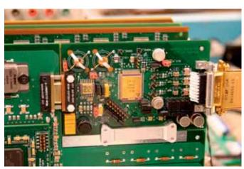
Engineering model of DFG electronics with space qualified Magnetometer Front-end ASIC in the middle (golden lid).
