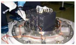
Vibration test of the MMO common instrument electronics box.
