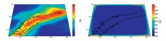
Geoid heights (a) and standard deviations (b) for the Novaya Zemlya area, derived from least squares collocation of gravity anomalies combined with GOCE gradients (simulated from EGM2008 D/O 50 to 2190, resp. 250).
