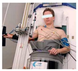
The Institute's Automated Multi-Stimulation Test Device for freely adjustable, automated, combined change of pitch (+70° head-up to -70° head-down tilt) and yaw (+30° to -30° sidewards slant). An additional lower body pressure system allows for POSUP experiment runs.
