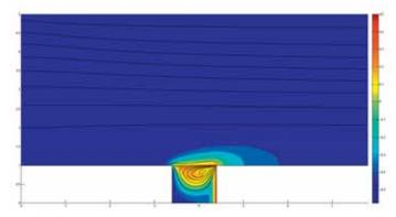
Steady streamlines and temperature field (colour) in a liquid bridge and in the exterior gas phase for a closed gas compartment (Fig. left) and for an open gas phase with imposed axial through flow (Fig. right). The cylindrical axis of symmetry is at the bottom of the figures.
