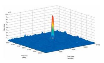
SoftGNSS acquisition result using a digital IF input signal
