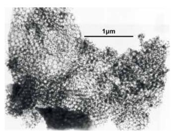
Macroporosity of the sol-gel films (from templating with polystyrene spheres).
