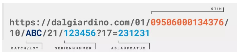
Figure 23: Example for GTIN integration in GS1
