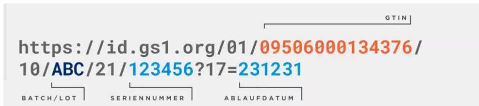
Figure 24: Example for extended GTIN integration in GS1
