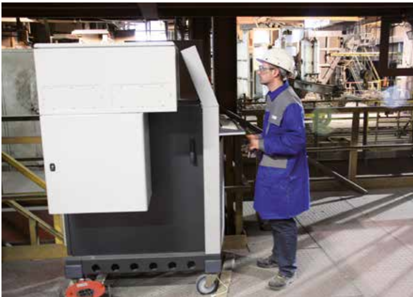
Analyzing the quality of slag in the voestalpine Stahl GmbH steel mill using a LIBS device from the Johannes Kepler University, Linz
